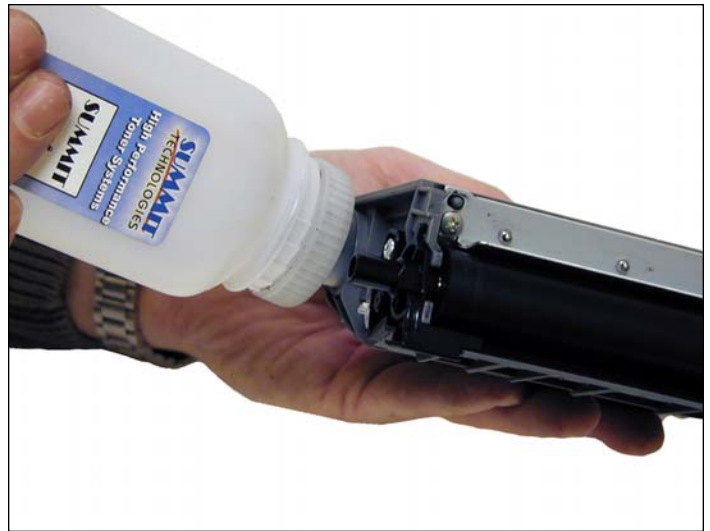
21. Fill the cartridge with Brother 2170 Black Toner
