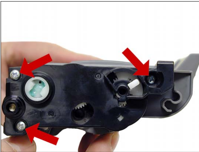
20. Install the gear cover plate, and three screws.
