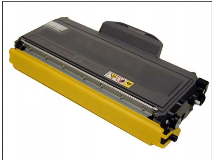
24. Install the developer roller cover.
